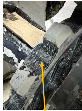
Sprocket Tooth Scoring
