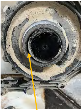
Idler Bearing Wear
