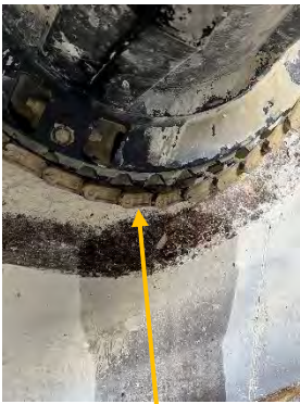
Idler Bearing Wear
