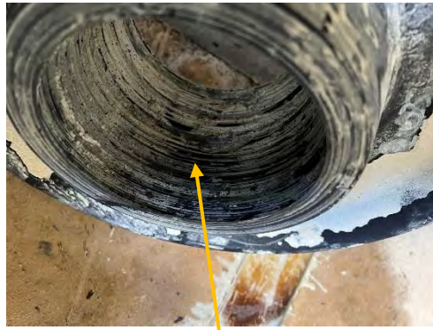
Sprocket ID Heavy Scoring
